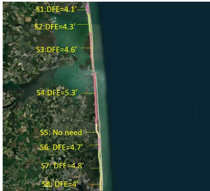
Figure 3-13: DFE of Raised Embankment for 10-year Event under the Current Condition with Structure Safety Criteria
