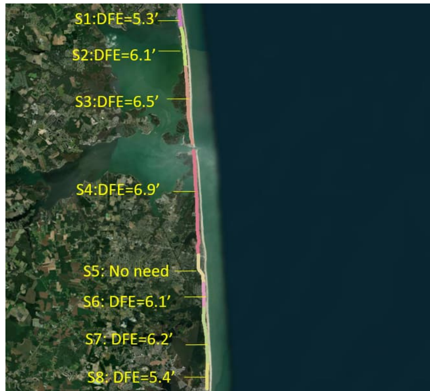
Figure 3-17: DFE of Raised Embankment for 100-Year Event under the Current Condition with Structure Safety Criteria
