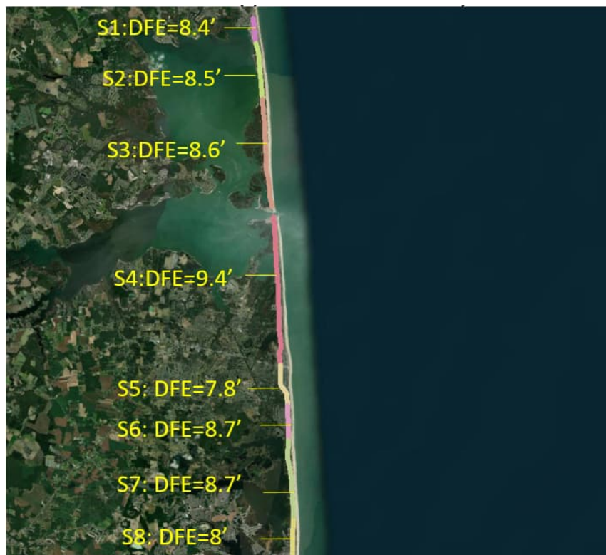
Figure 3-16: DFE of Floodwall for 100-Year Event with the SLR in 2075 with Structure Safety Criteria
