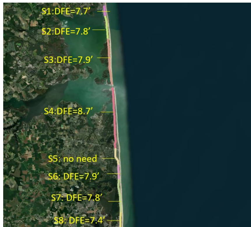
Figure 3-14: DFE of Raised Embankment for 10-Year Event with SLR in 2075 with Structure Safety Criteria
