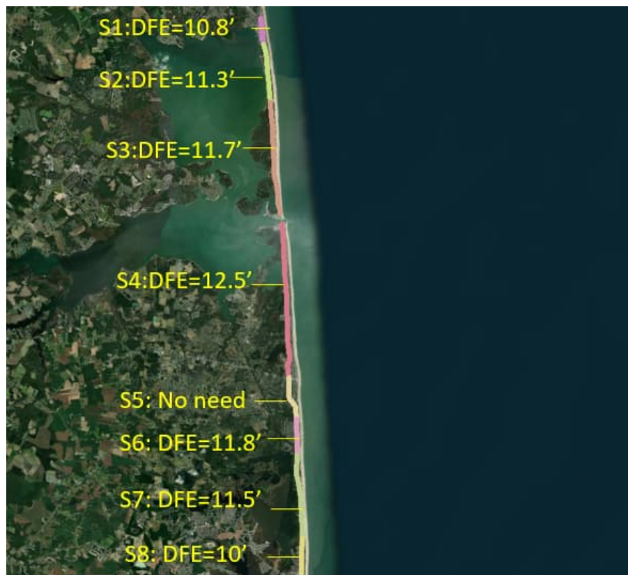
Figure 3-19: DFE of Floodwall for 100-Year Event with the SLR in 2075 for Driving Safety Criteria
