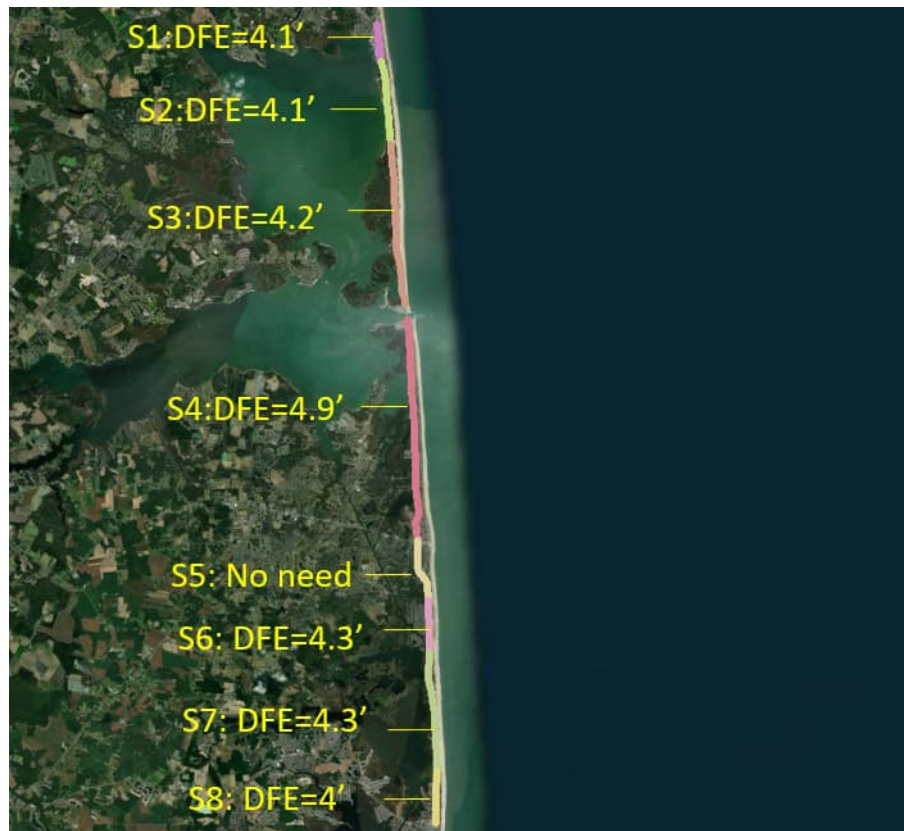
Figure 3-11: DFE of Floodwall for 10-year Event under the Current Condition with Structure Safety Criteria
