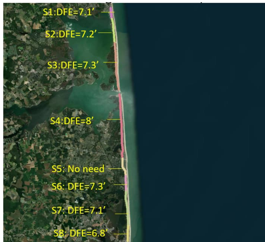
Figure 3-12: DFE of Floodwall for 10-Year Event with SLR in 2075 with Structure Safety Criteria
