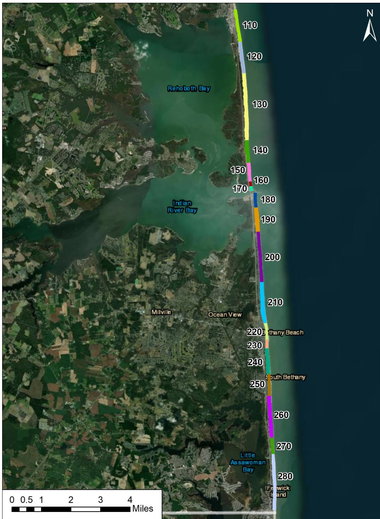
Figure 3-6: Location of 18 Shoreline Segments Used in Sediment Transport Analysis
