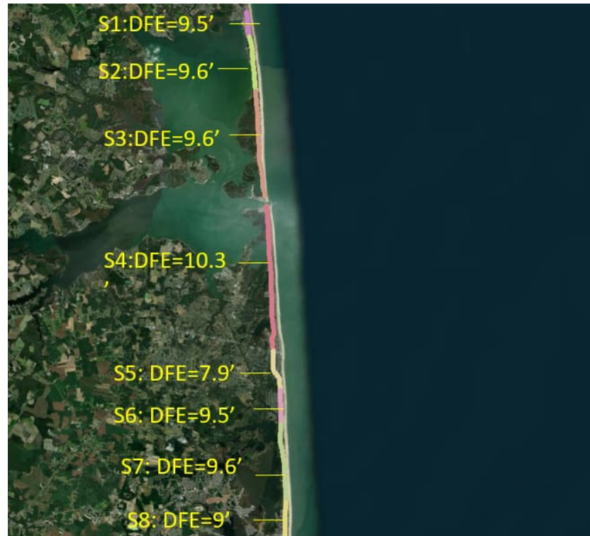
Figure 3-18: DFE of Raised Embankment for 100-Year Event with the SLR in 2075 for Structure Safety Criteria
